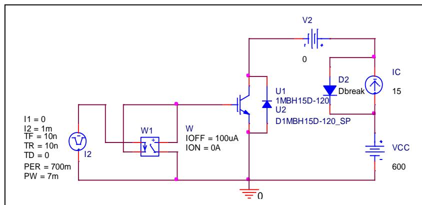
Test condition:  $V_{CC}=600$  (V),  $I_C=15$  (A),  $V_{GE}=15$  (V)
