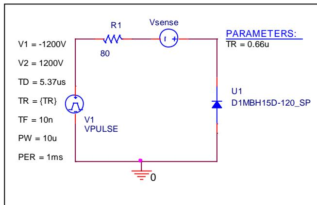
Test condition:  $Vcc=1200$  (V),  $Ic=15$  (A),  $-di/dt=45$  (A/ $\mu$ s)
