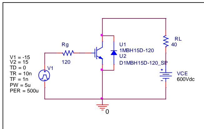
Test condition:  $I_C=15$  (A),  $V_{CC}=600$  (V)
